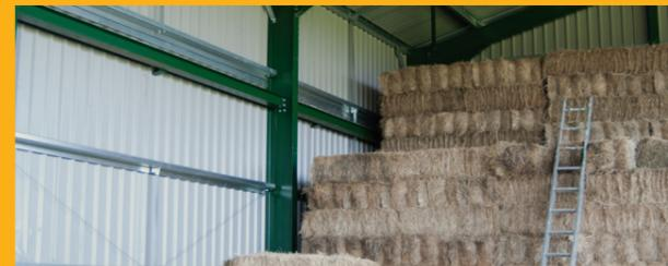
The crops need to be kept cool and dry. Eternit sheets can help with this as they not only have good thermal performance to keep the heat from outside at bay, they also retain moisture to reduce the chance of any dripping on the crops.
